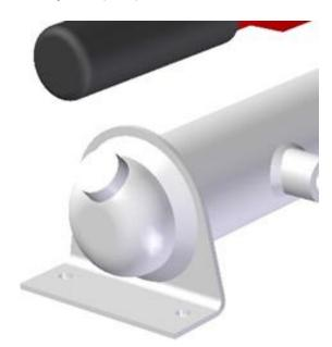
Ensure that the filler plug seal is not damaged or missing, as this acts as the safety valve to prevent over-pressure in the system. Replace the filler plug.
